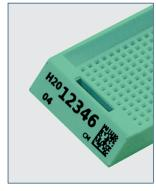
Thermal transfer print quality delivers a durable, high-contrast print, protected during dewaxing by pips on the corners of the cassettes.
